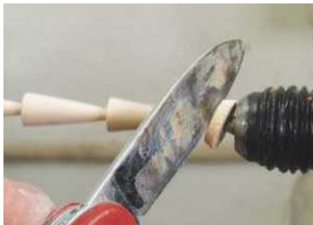
▲ Pic.8 Removing the waste from the tailstock with the lathe running is best done with a skew. Turn the lathe off and cut off using a pen knife, but be careful not to pull out the fibres
